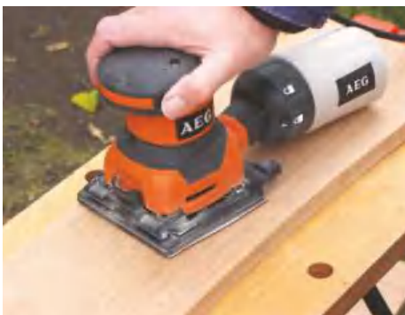
STEP 10. Sand the back panel and underside of the shelf before gluing the rack together
